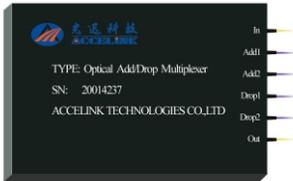
Optical add/drop Multiplexer are available on ITU channel spacing of 100GHz, 200GHz, and 20nm, they are based on thin film filter technology and flexible integration of taps and detectors for a complete wavelength division multiplexing solution. The products adopt hermetic package craft and environmental stability. The products are Telcordia GR-1221-CORE qualified, and RoHS compliant.
